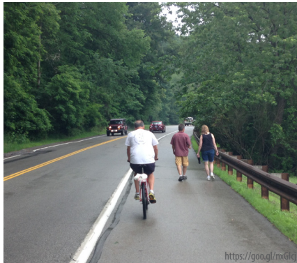
Figure 3-1. A striped shoulder can be a low cost corridor good for road segments without frequent stop or signaled intersections.
